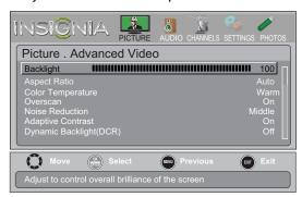
Backlight—Sets the overall brilliance of the screen. When Dynamic Backlight (DCR) is turned on, you cannot change the Backlight setting.  Aspect Ratio—Selects the aspect ratio of the picture.
